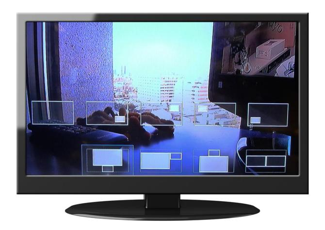
Choose from an assortment of screen layouts that incorporate the self-view window in various positions and sizes. To hide the self-view window, navigate to the Layout option and select the single rectangle.
